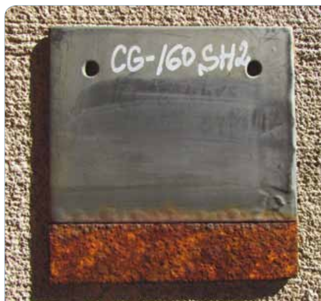
Figure 4. Exposed border corroded, no undercut disbondment.
