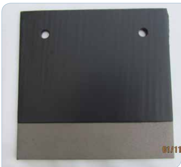
Figure 3. New test plate coated with CorrosionGard™ 160SH2.
